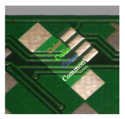
utilization. Different types of RGB LED's can be used on each output, the only requirement is that all LED's must be the same polarity type (common +/-). The common connection goes to the common pin of the LED and the 3 color connections can be made in any configuration, BUT all need to be connected the same way. All red light elements must be connected to the same position across all LED outputs, etc.
